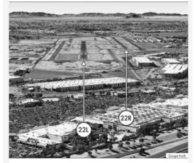
Offset parallels; RWY 22R is 2190 feet farther down the approach than RWY 22L; a rectangular building on 1/2 mile final is aligned with RWY 22R.
