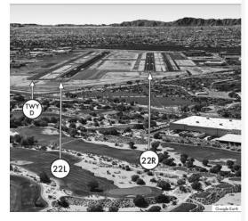
Offset parallels; RWY 22R is 750 feet farther down the approach than RWY 22L. Pilots sometimes confuse RWY 22L and Runway 22R, or TWY D for RWY 22L.
