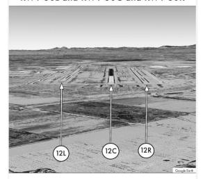
Offset triple-parallels; RWY 30L is offset from RWY 30C and RWY 30R. RWY 30L is 1300 feet farther down the approach than RWY 30C and RWY 30R.
