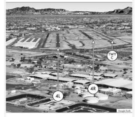
Offset parallels; RWY 4R is 1700 feet farther down the approach than RWY 4L. Pilots confuse RW 4L and RWY 4R, and TWY C for RWY 4R.
