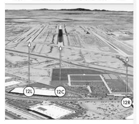
Offset triple-parallels; Pilots sometimes confuse RWY 12L or RWY 12R for RWY 12C, and RWY 12R or RWY 12C for RWY 12L.
