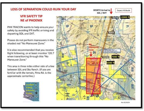
The Carefree area is such a hazard area. The area between the two red lines should be a non-maneuvering area. <u>Cary Grant:</u> Bob Mittelstaedt has been working on a new graphic to help pilots understand the Carefree area and what to avoid, and here it is! This graphic is a suggestion, not a requirement. Cary asked Bob to shade the area translucently.
